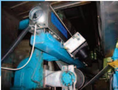
refrigerated air and double casings are used to enable a trouble free operation even in demanding press section applications. Standard features include a fast response time (2.5ms), a very long service interval (about 20 years) and a wide moisture range (0-70%). The sensor operates with Near Infrared fixed filters and obtains its sensor reading simultaneously (same-spot measurement).
