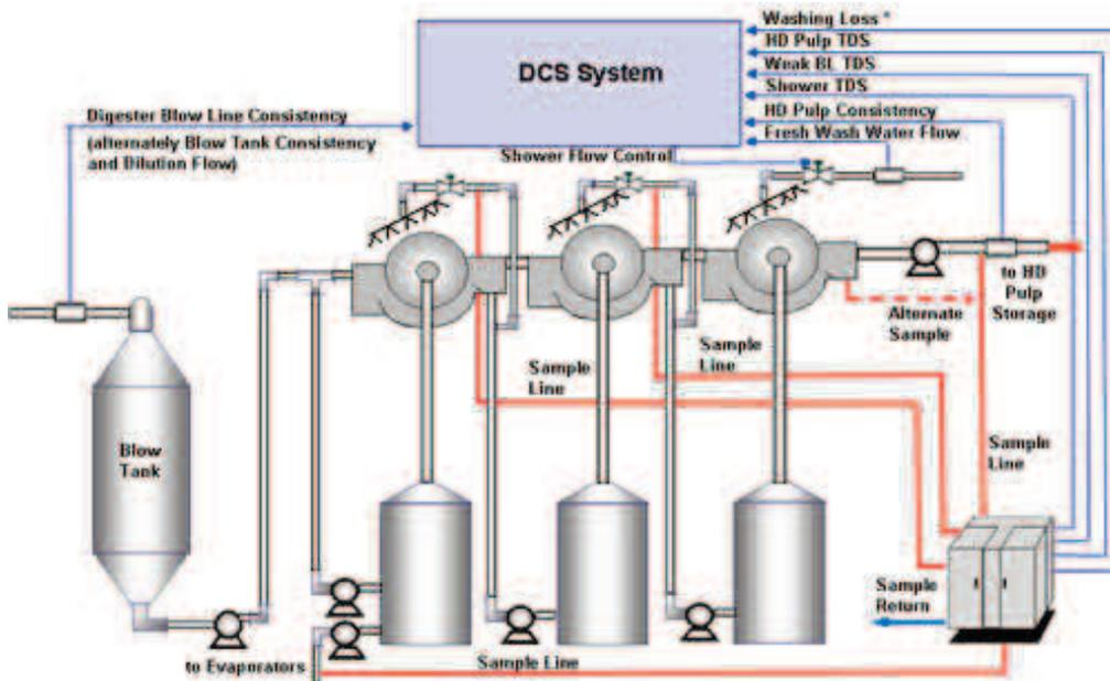
**THE UNIQUE DESIGN** of this analyzer has proven itself in several other difficult Kraft Pulping and Recovery applications to be practically maintenance free, physically small and portable with easy installation and low installed cost. Specific attention to design details have eliminated problems associated with collecting samples..
