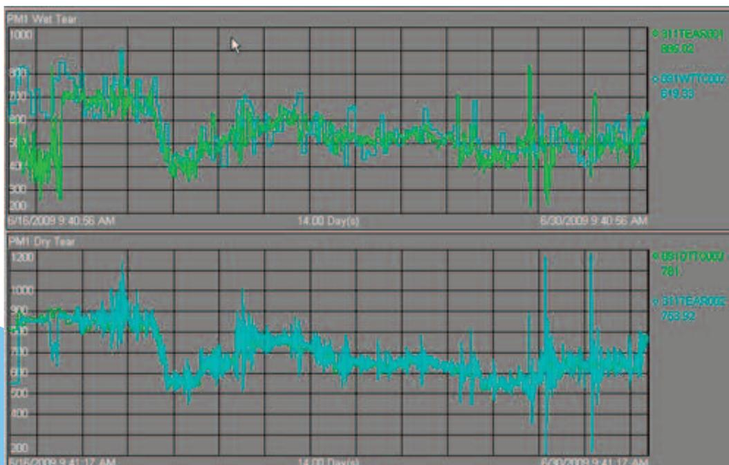
**TO THE RIGHT** is a typical operator display, showing the actual predicted value (updated every minute) along with a horizontal bar indicating the direction in which the tear is shifting. An eight hour tear trend is also displayed.
