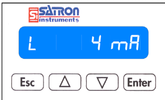
Figure 2-4 VDt differential pressure transmitter with display
